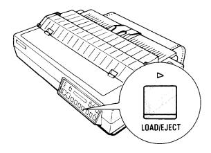
**Note:** If you press **the LOAD/EJECT** button when continuous paper is **already loaded**, **the paper is reversed to the standby** position.
